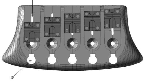
Over here you hook up the string. When putting on a new string, always make sure not to twist it around its axis.
